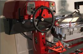
This extra length on the beam (optional) is available to ease the mounting and unmounting of large and heavy cylinder heads on the floating table.
