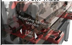
Cylinder heads up to 350 kgs can be moved back and forth without any effort and then locked by two powerful pneumatic jacks.
